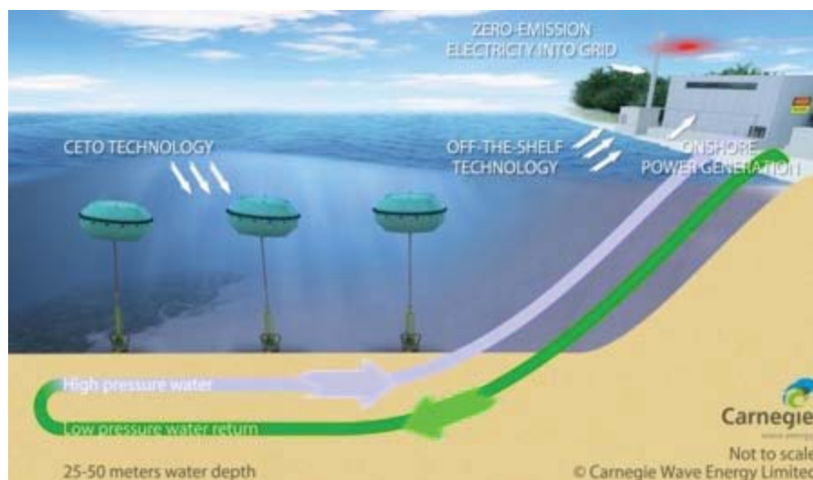
Figure 1. CETO technology schematic
